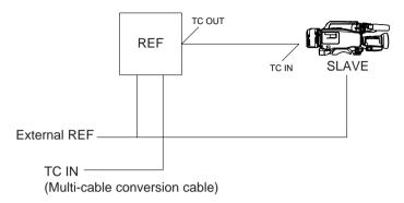
Example 2: Connecting multiple units and using one unit as the reference
